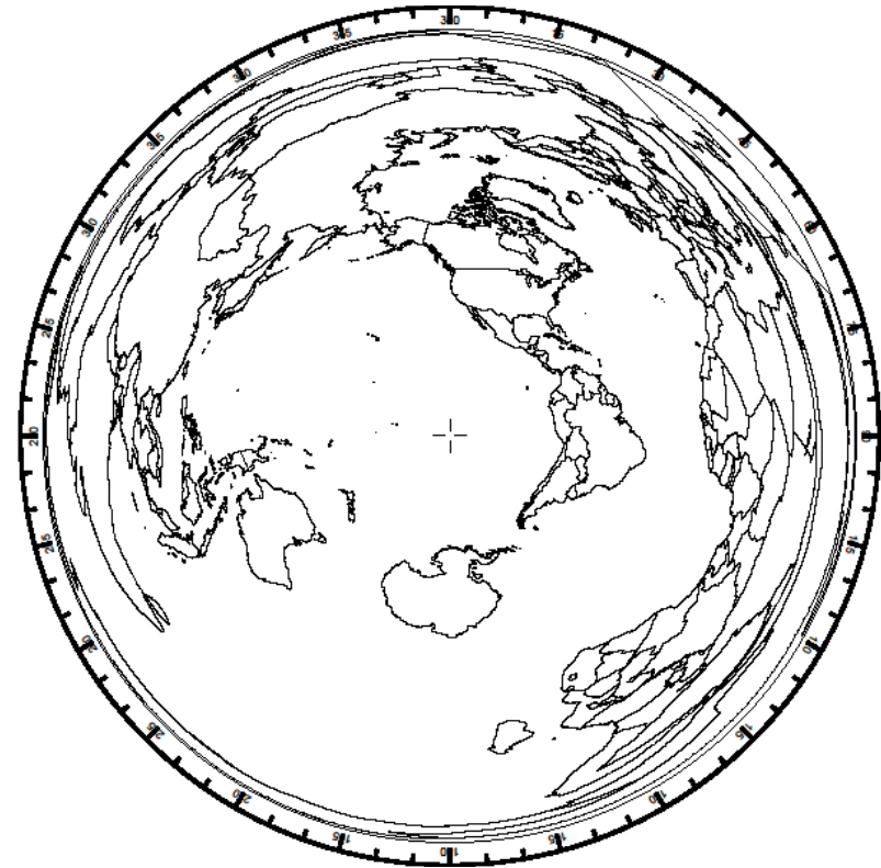
Figure 1: Eq-az (great circle) chart centered on Ducie Island. Note that short path signals to Europe and west Asia cross over North America. Sector divisions on this map illustrate the ranges of azimuths covered by the eight receiving antenna beams available to the Ducie Island low-band operators.
