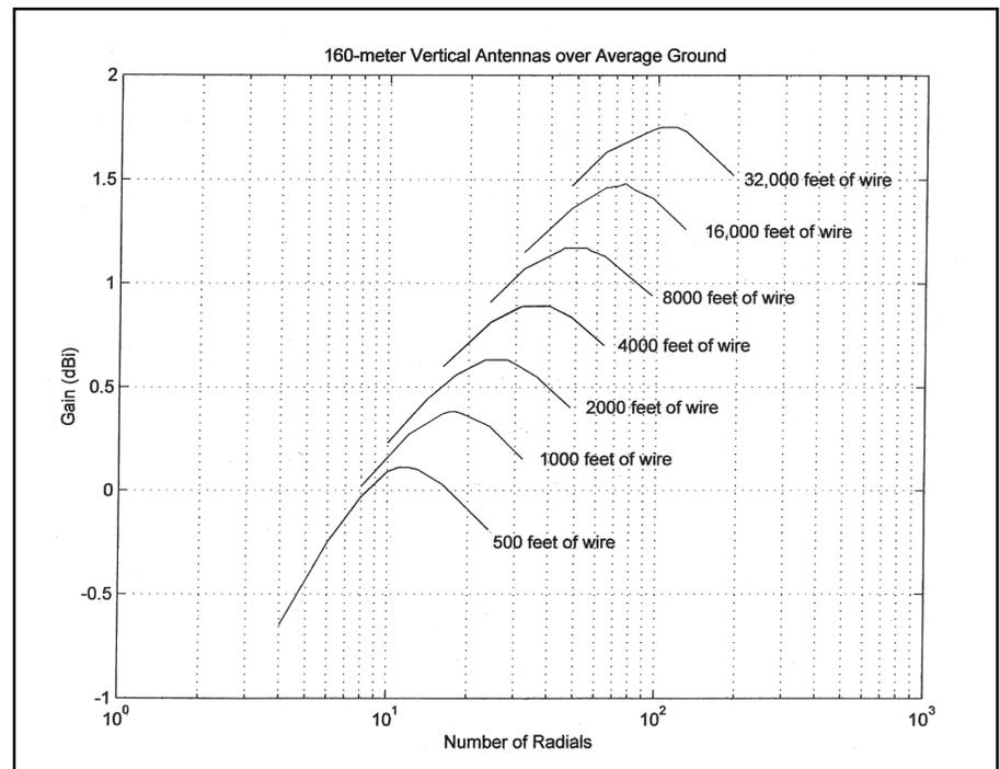
**Figure 3—Gain of a quarter-wave 160 meter vertical antenna over average soil, as the number of buried radials is varied, for seven different total lengths of wire.**
