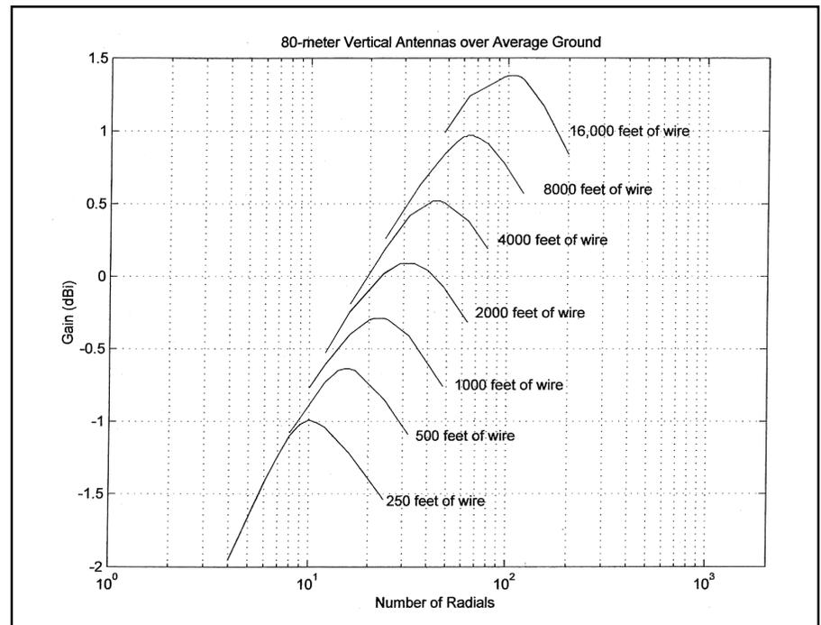
Figure 2 — Gain of a quarter-wave 80 meter vertical antenna over average soil, as the number of buried radials is varied, for seven different total lengths of wire.
