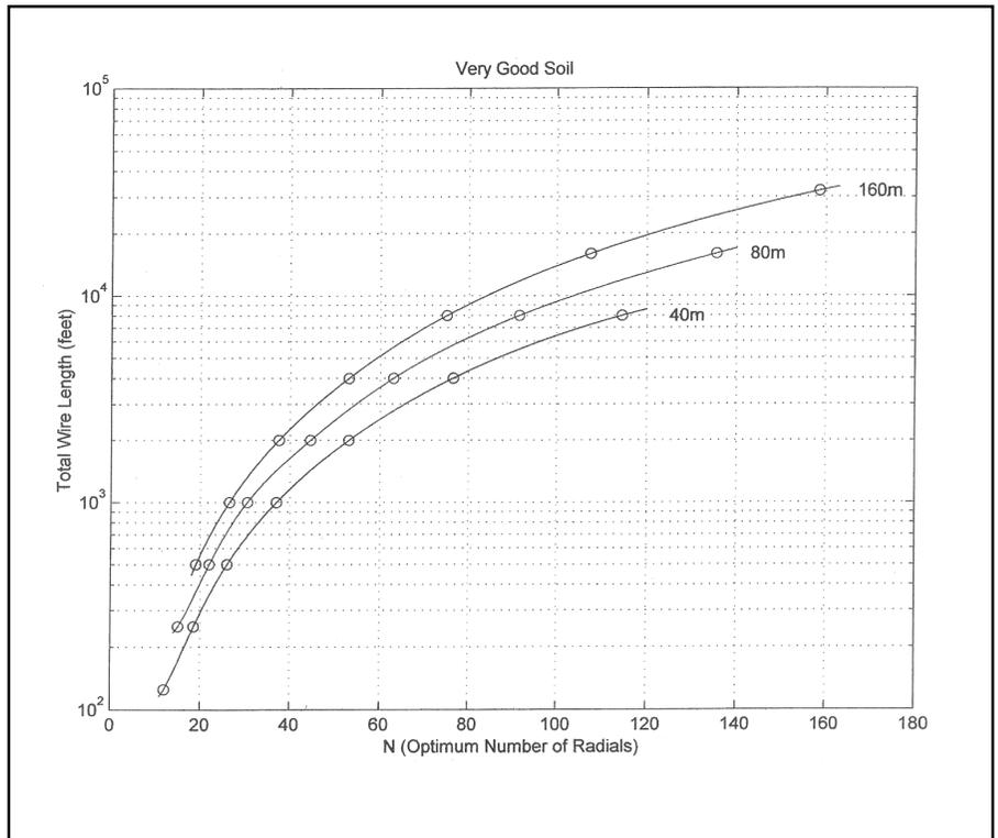
**Figure 6—Optimum number of buried radials for quarter-wave vertical antennas over very good soil, as the total wire length is varied, for the three “low bands” 40, 80, and 160 meters.** NCJ
