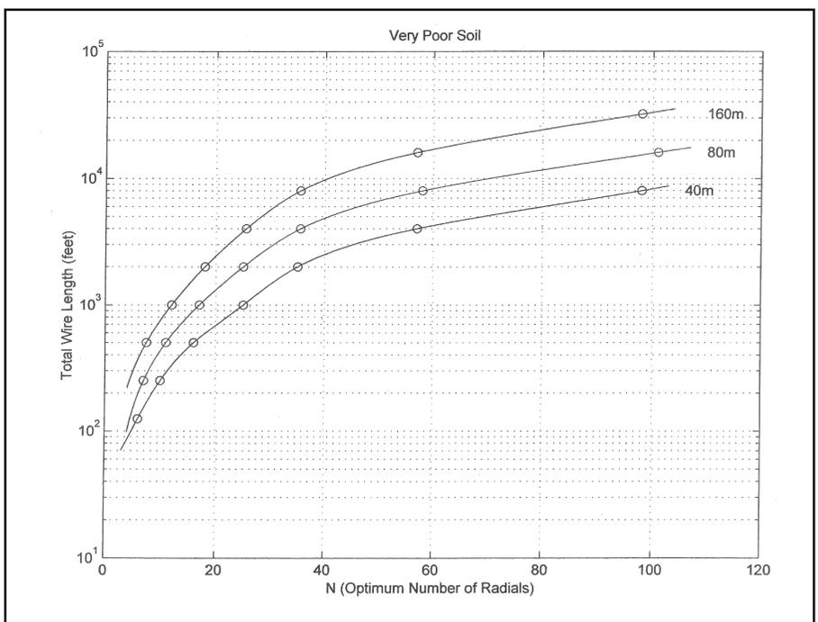
**Figure 5—Optimum number of buried radials for quarter-wave vertical antennas over very poor soil, as the total wire length is varied, for the three “low bands” 40, 80, and 160 meters.**
