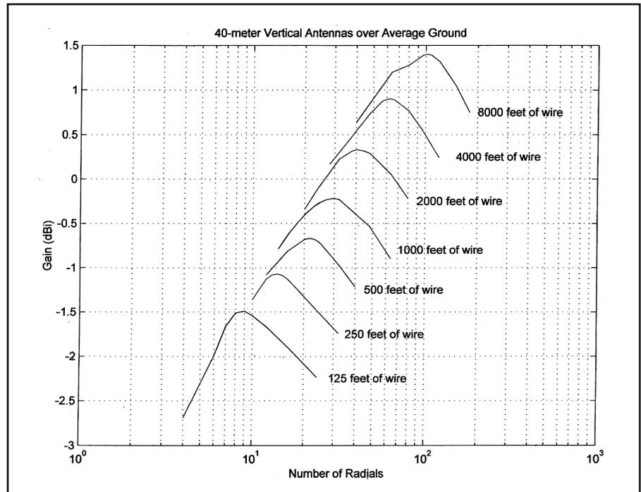
Figure 1—Gain of a quarter-wave 40 meter vertical antenna over average soil, as the number of buried radials is varied, for seven different total lengths of wire.
